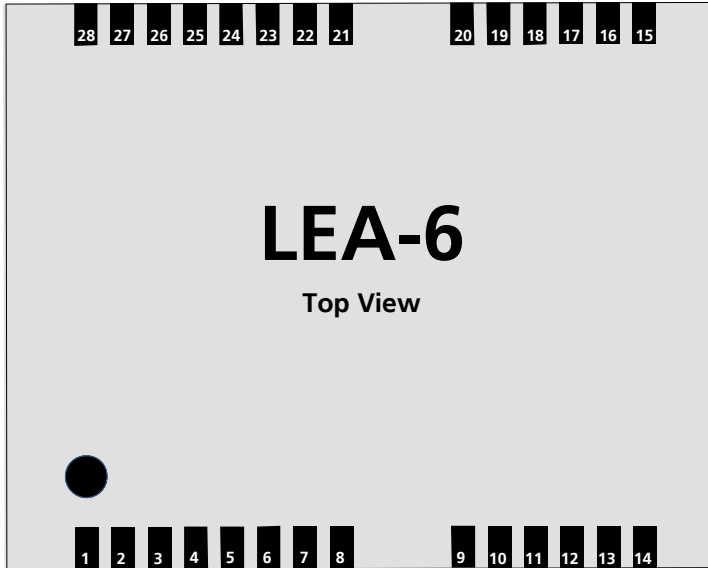
Figure 2 LEA-6 Pin Assignment
